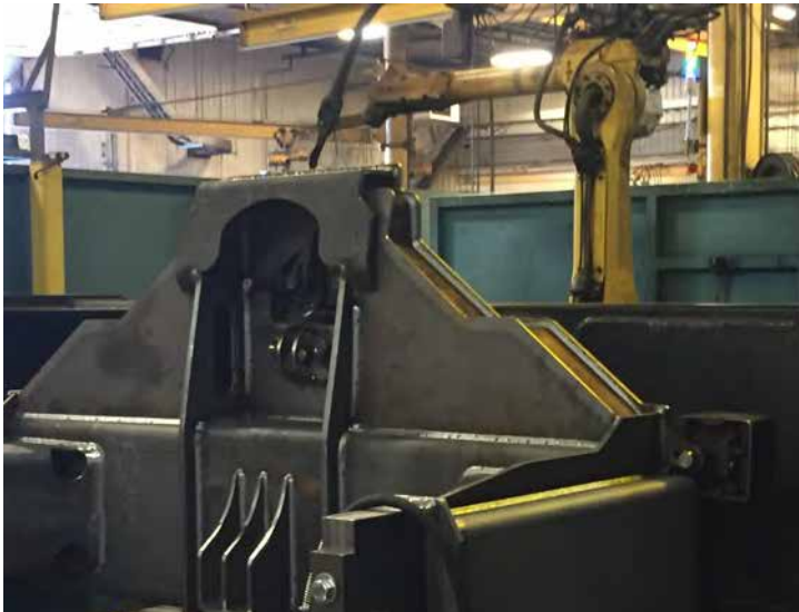
Small Robotic Welder
